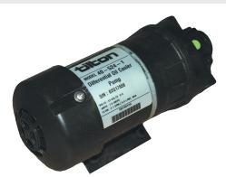
dition with a more typical current draw between 2 and 3 amps. This pump has a very light weight at 3.5 lbs and has a flow rate of 1-2 gallons per minute. There are two types of diaphragms available for the differential pumps; the BUNA type diaphragms are for standard coolants and the VITON diaphragms are for the more corrosive coolants.
